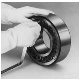
Fig. 1: Checking bearing clearance with bearing on bench.
