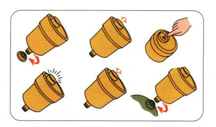
To start the **PULLARLUBE**, depress the button located beneath the screw-on, clear waterproof cap. Once activated, a green indicator lamp flickers 7 to 8 seconds to confirm operation. As long as the lamp is illuminated, the unit is working.
